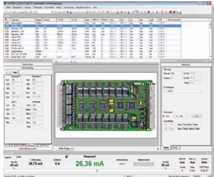
Programming PSUs in the function test form
