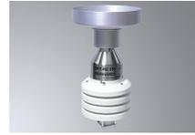
**Combi-Sensor DFT-RE 55Y** measures temperature, humidity, barometric pressure and precipitation, 200 cm<sup>2</sup> collecting area, 5 free analog inputs, RS232-data output (optional: RS422, USB, TCP/IP, PoE, WLAN etc.), 32 GB data logger, PC-software for display, control and evaluation
