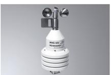
**MWS 55Y Weather Station** measures temperature, humidity, barometric pressure, wind direction, wind speed, 5 free analog inputs and 1 free TTL-input, RS232-data output (optional: RS422, USB, TCP/IP, PoE, WLAN etc.), 32 GB data logger, PC-software for display, control and evaluation
