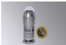
**GSS 485 Global Radiation Sensor** measures global radiation (305 to 2,800 nm) from 0 to 1,500 W/m<sup>2</sup>. 73 mm high with glass hemisphere and housing, 25 mm diameter; power supply 6–30 VDC, with RS232-data output (optional RS422 or RS485), without software, power supply and cabling
