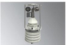
**MWS 88-2Y Microprocessor Weather Station**, measures temperature, humidity, barometric pressure, wind direction, wind speed, 5 free analog inputs and 1 free TTL-input, RS232-data output (optional: RS422, USB, TCP/IP, WLAN etc.), 32 GB data logger, PC-software for display, control and evaluation
