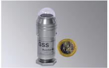
**GSS Analog Global Radiation Sensor** measures global radiation (305 to 2,800 nm) from 0 to 1500 W/m<sup>2</sup>. 76 mm long with glass hemisphere and housing, 25 mm diameter; cable connection with 3 wires (ground, supply voltage from 5V or 8–20 VDC and output signal from 0–4V).
