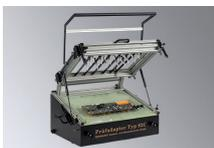
**Manual Test Fixture Type 82C** 4 linear guidings, 2 x 18VG-interface, exchange plate (FR4), working area 480x320mm, overall dimensions of the plate 500x400x8 mm, exchange
