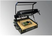
**Manual Fixture Type 42A**, 4 linear guidings, hinged upper part, exchange plate (CEM1), working area 360 x 230 mm, overall
