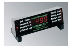
**DKA1 Digital Meteo Display** for MWS-weather stations, dimensions 6 x 14.5 x 5.5 cm, with 9 alternating digital LED-displays (red, 7 segment). A blinking parameter is the measured value. 4 positions, character height 13.2 mm, without plug-in supply (can be supplied straight from the weather station), for indoor use
