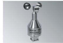
**Wind Speed Sensor WGS 55Y** measures wind speed, average wind and gust speed, 5 free analog inputs and 1 free TTL-input, RS232-data output (optional: RS422, USB, TCP/IP, PoE, WLAN etc.), 32 GB data logger, PC-software for display, control and evaluation, without power supply and cabling
