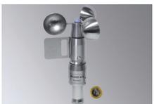
**Miniature Combi-Sensor WGWR 485** measures wind speed, gust speed and wind direction, power supply 6–30 VDC, with RS232-data output (optional USB, TCP/IP, WLAN, GSM) incl. software for display, control and evaluation; without power supply and cabling
