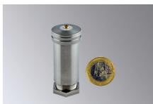
**UVIS 485 Ultraviolet Sensor** for direct measurement of the UV-index from 0–12 (UV radiation intensity relevant to sunburn), erythemal action spectrum. 65 mm high, diameter 25 mm. Power supply 6–30 VDC, with RS232-data output (optional RS422 or RS485), without software, power supply and cabling
