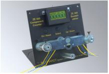
**ZE 300 Component Counter** for radial, axial and SMD-banded components, incl. NC-rechargeable battery and charger. Independent of mains supply, microprocessor controlled, preset number of pieces and separation mark, adjustable display. Tape width of SMT-components can be set from 8 mm to 60 mm; optional RS232-interface
