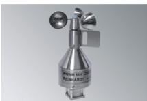
**Combi-Sensor Wind WGWR 55Y** measures wind speed, gust speed and wind direction, 5 free analog inputs and 1 free TTL-input, RS232-data output (optional: RS422, USB, TCP/IP, PoE, WLAN etc.), 32 GB data logger, PC-software for display, control and evaluation
