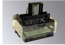
**Pneumatic Fixture Type 40A**, 4 linear guidings, with voltage supply, dual stage retention (in-circuit- and function test), with exchange plate
