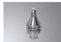
**Global Radiation Sensor GSS 55Y** measures solar energy (305 nm to 2800 nm) with a pyranometer, 0 to 1300 W/m<sup>2</sup>, 5 free analog inputs and 1 free TTL-input, RS232-data output (optional: RS422, USB, TCP/IP, PoE, WLAN etc.), 32 GB data logger, PC-software for display, control and evaluation, without power supply and cabling
