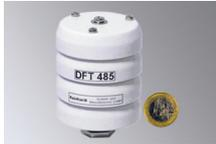
**Combi-Sensor DFT 485** measures temperature, relative humidity, dew-point and barometric pressure, head diameter about 60 mm, 86 mm high, power supply 6–30 VDC, with RS232-data output (optional RS422 or RS485) incl. software for display, control and evaluation; without power supply and cabling
