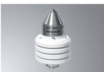
**Combi-Sensor DFT 55VY** measures temperature, humidity and barometric pressure, 5 free analog inputs and 1 free TTL-input, RS232-data output (optional: RS422, USB, TCP/IP, PoE, WLAN etc.), 32 GB data logger, PC-software for display, control and evaluation
