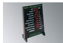
**DMMK Small Digital-Meteo Multi Display** for MWS-weather stations, dimensions without foot about 30 x 20 x 2.8 cm, with up to 12 simultaneous digital LED-displays (red, 7 segment), 4 positions, height of characters 13.2 mm, RS232-interface, optional TCP/IP and WLAN, incl. AC-plug-in supply, for indoor use
