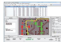
**RDR Off-line Repair Station** for repair, with precise graphical display of faults, use of the statistics data by module
