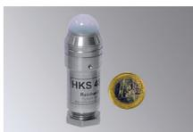
**HKS 485 Global Radiation Sensor** measures light intensity from 0 to 220,000 Lux. 73 mm high with glass hemisphere and housing, 25 mm diameter; power supply 6–30 VDC, with RS232-data output (optional RS422 or RS485), without software, power supply and cabling
