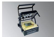
**Manual Test Fixture Type 127** working area 191.5x172 mm, with lower exchange plate (CEM1), overall dimensions of the plate 217.6x230x8 mm,
