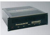
**POMO80 Power Module** with 1 DC-source max. 80V, 14A, 2 loads max. 100V, 30A, 1mA, total power up to 1,000W, RS232-interface, ramp
