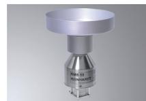
**Precipitation Sensor RMS 55Y** measures precipitation with a self-emptying bucket, 200 cm<sup>2</sup> collecting area, 5 free analog inputs, RS232-data output (optional: RS422, USB, TCP/IP, PoE, WLAN etc.), 32 GB data logger, PC-software for display, control and evaluation, without power supply and cabling, heating optional
