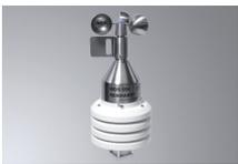
**Combi-Sensor Wind WTF 55VY** measures temperature, humidity, wind speed, gust speed and wind direction, 5 free analog inputs and 1 free TTL-input, RS232-data output (optional: RS422, USB, TCP/IP, PoE, WLAN etc.), 32 GB data logger, PC-software for display, control and evaluation
