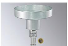
**RMS 485 Precipitation Sensor** measures precipitation with a self-emptying bucket and a collector vessel with 200 cm<sup>2</sup>, 170 mm high; Power supply 6–30 VDC, with RS232-data output (optional RS422 or RS485); without software, power supply and cabling
