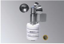
**MWS 3** measures temperature, relative humidity, barometric pressure, wind speed, gust speed and wind direction, voltage supply 6–30 VDC, with RS232-data output (optional RS422, RS485, USB, TCP/IP, WLAN etc.), PC-software for display, control and evaluation, without power supply and cabling
