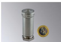
**WKS 485 Sensor for Detection of Cloudiness** ascertains independent of sun or moon if there is a cloud layer. From the measured values the height of cloud base can be found. 63 mm high, diameter 25 mm. Power supply 6–30 VDC, with RS232-data output (optional RS422 or RS485), without software, power supply and cabling
