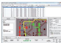
**RUDC10 Universal Data Converter** (CAD-interface) for REINHARDT-Windows-test systems for import of components data and coordinates of
