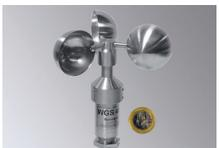
**WGS 485 Wind Speed Sensor** measures wind speed 0–200 km/h, resolution 0,05 km/h, average wind, gust speed. 115 mm high, diameter anemometer 120 mm. Power supply 6–30 VDC, with RS232-data output (optional RS422 or RS485), without software, power supply and cabling.
