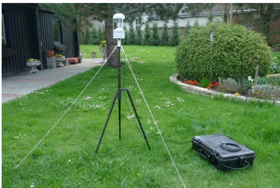
For unsupervised operation you can close the case and run the system without computer at the connector at the case.
