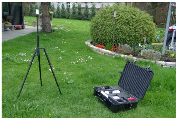
Then the weather station is mounted on top of the tripod, orientated to north and fixed on the tripod with the 2 screws at the socket. Please take care that the tripod stands fixed on the ground to avoid dropping of the tripod in case of wind. With internal cabling you may run a laptop in parallel to the measurement.
